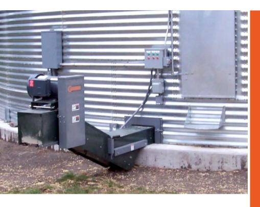
These conveyors are used under the aeration floors of grain bins.
