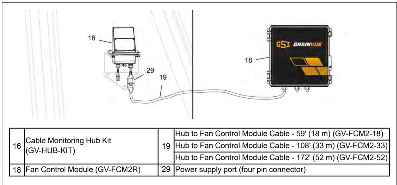
8. Capture a picture or document the Cable Monitoring Hub (16) S/N that is located on the label found on the back face of the Hub (16) to be used in the commission process. Refer to [Chapter 2, System Overview and Commissioning, page 15](#) for details.
