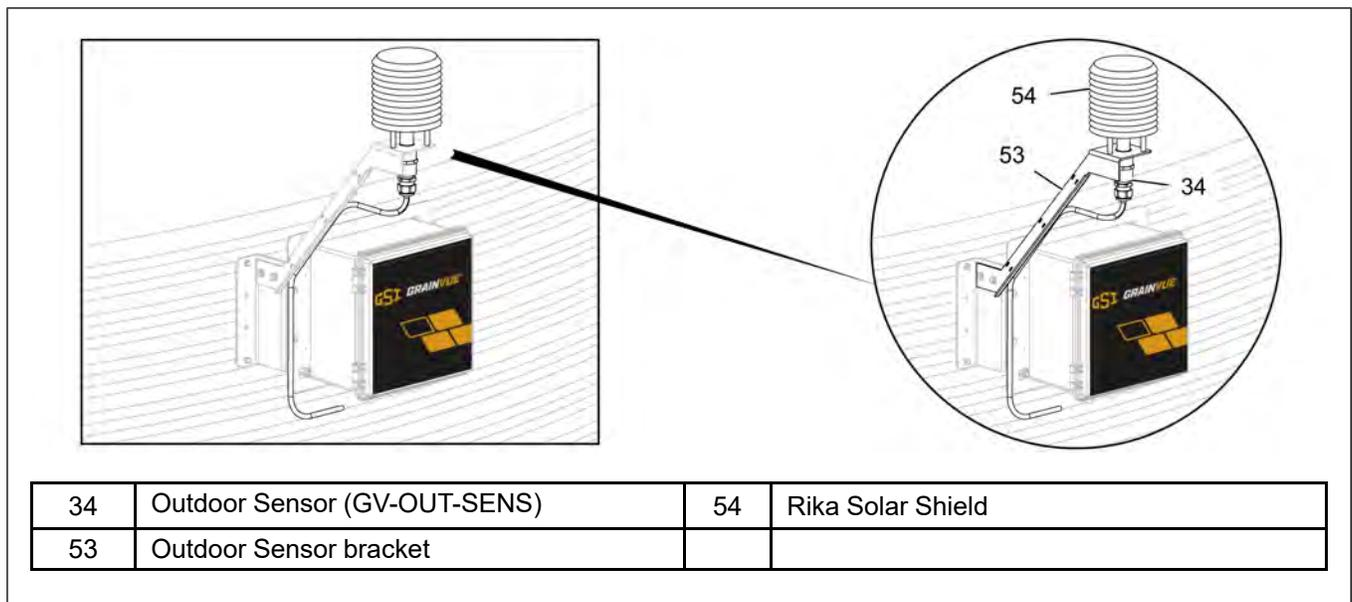
4. Use zip ties to secure the Outdoor Sensor cable (55) to the Outdoor Sensor bracket (53) using the slots on the bracket.
