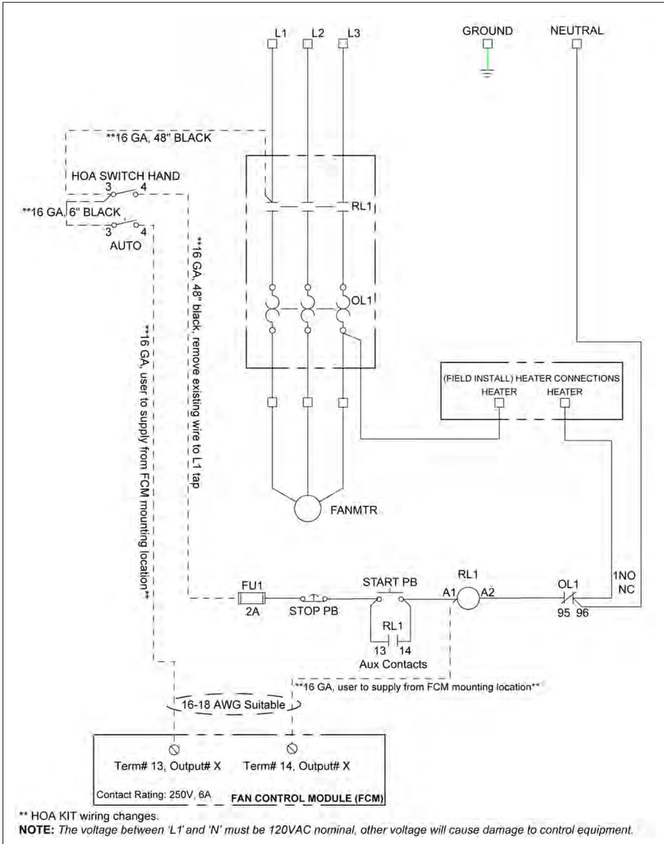
Figure 8-5 480 Volt 3 Phase - 120V control circuit
