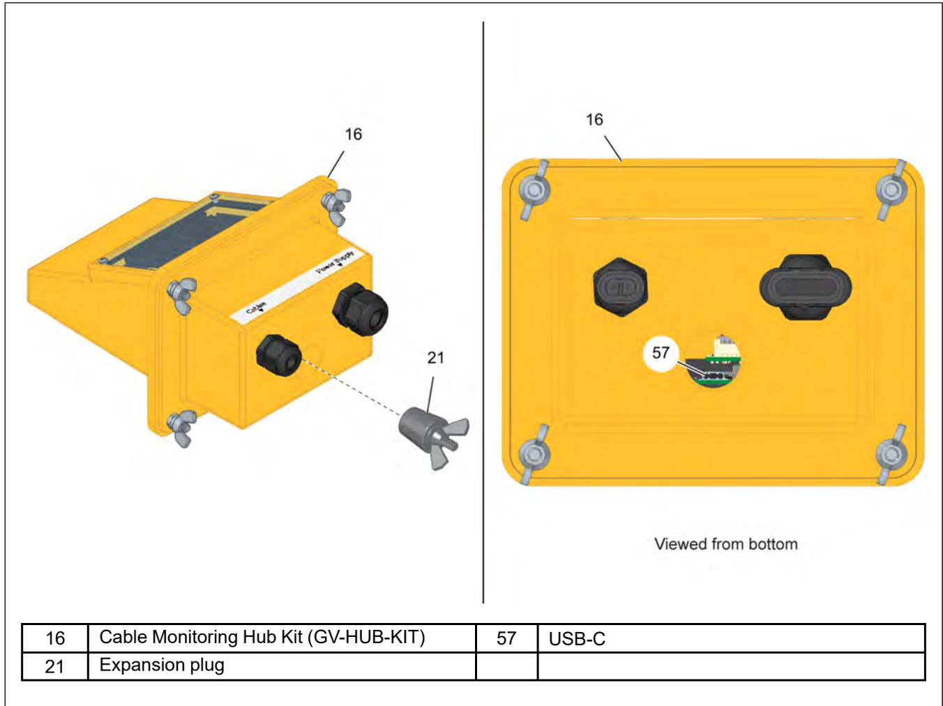
4. Turn the Hub (16) ON, refer to [Chapter 7, Activating the Cable Monitoring Hub, page 83](#) section of this guide.
