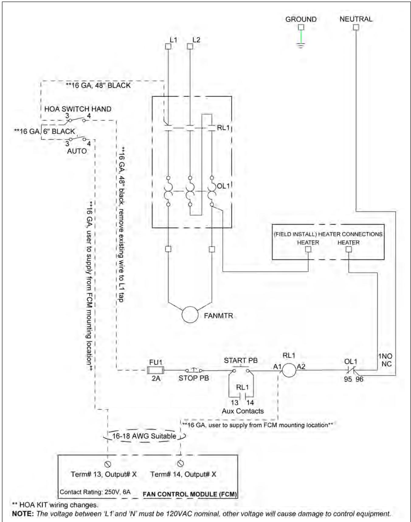
Figure 8-4 240 Volt 3 Phase - 120V control circuit
