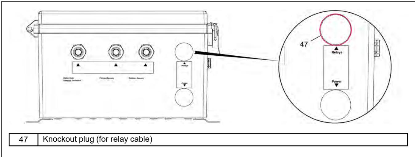
2. Connect the conduit to the Fan Control Module and run to each fan contactor box or fan control device.
