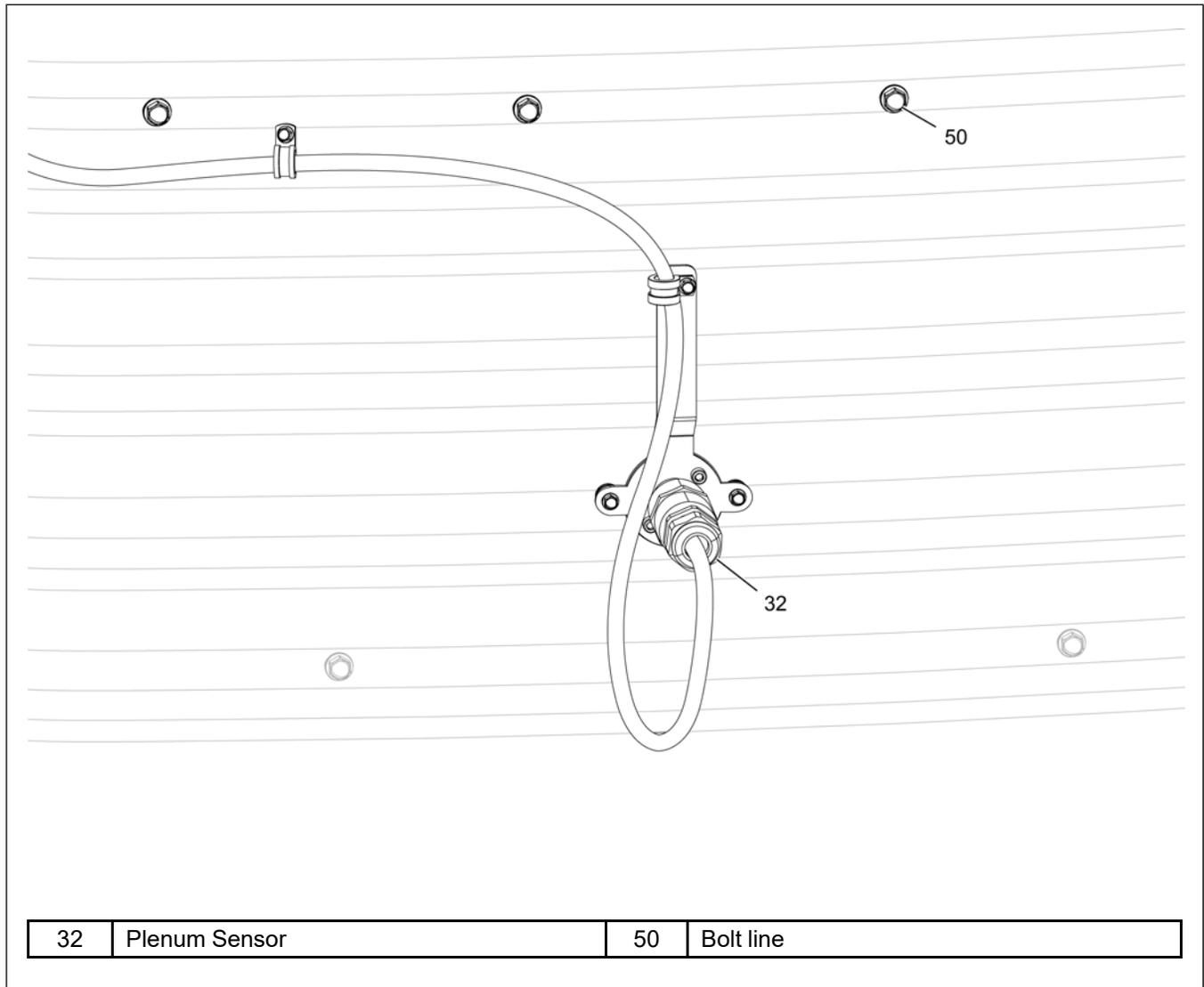
2. Insert the Plenum Sensor (32) into the 2-1/2" hole with the handle in the downward position if possible. The handle can go in the upward position if the sensor is too close to the foundation. Push the foam core of the Plenum Sensor (32) into the hole, sealing all edges of the hole.
