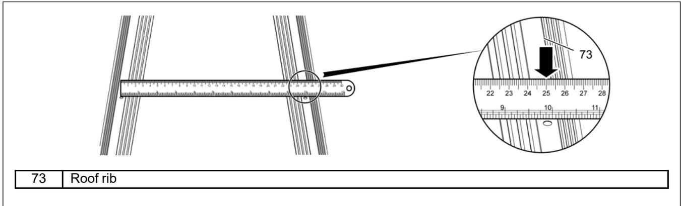
4. Drill a 1-1/2" hole with the hole saw at the marked point while angling the hole saw so that it is perpendicular to the roof panel (76) of the bin.
