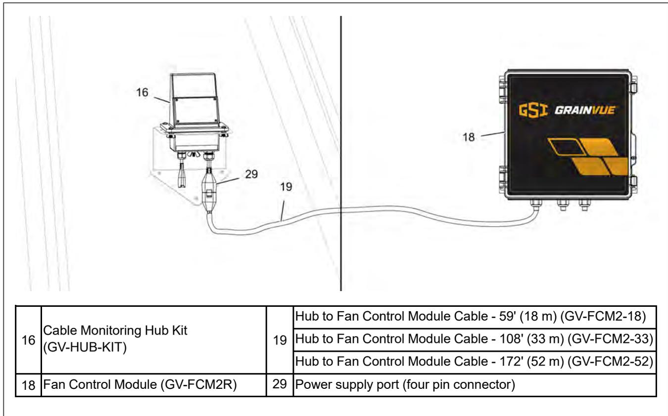
1. The free end of the cable (19) will enter the Fan Control Module (18) through the left most cord grip (43). Before running the cable (19) through the cord grip (43), excess length of cable (19) can be cut off. Do not cut the cable (19) too short, and leave a few feet of extra cable (19) should any re-work or re-routing be required.
