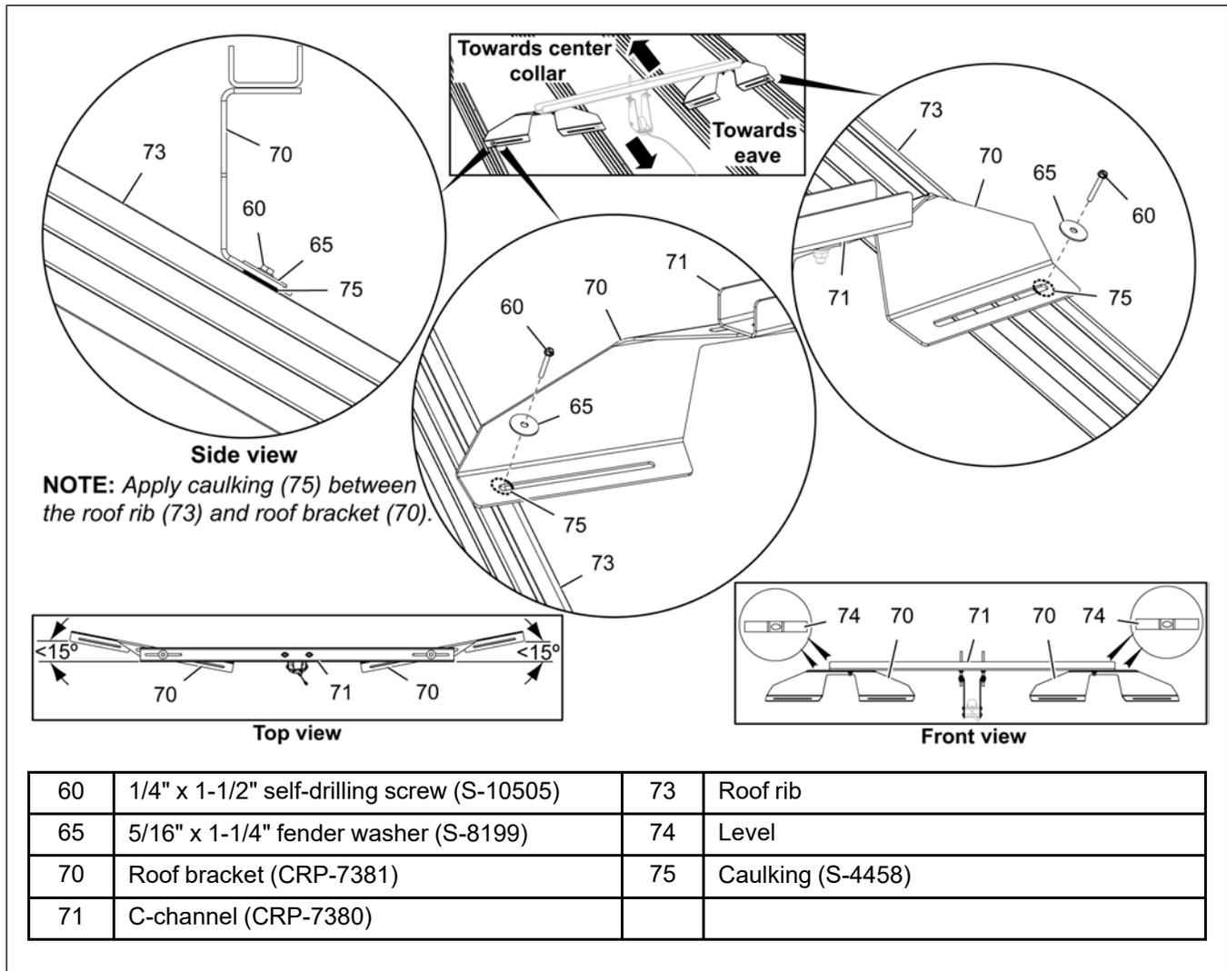
14. Tighten all the 1/4" x 1-1/2" self-drilling screws (60) securing the roof brackets (70) to the roof ribs (73). Tighten all the 3/8" x 1-1/4" HHCS bolts (61) securing the C-channel (71) to the roof brackets (70).
