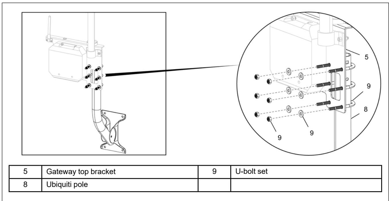
3. Install the cell communication antenna.
