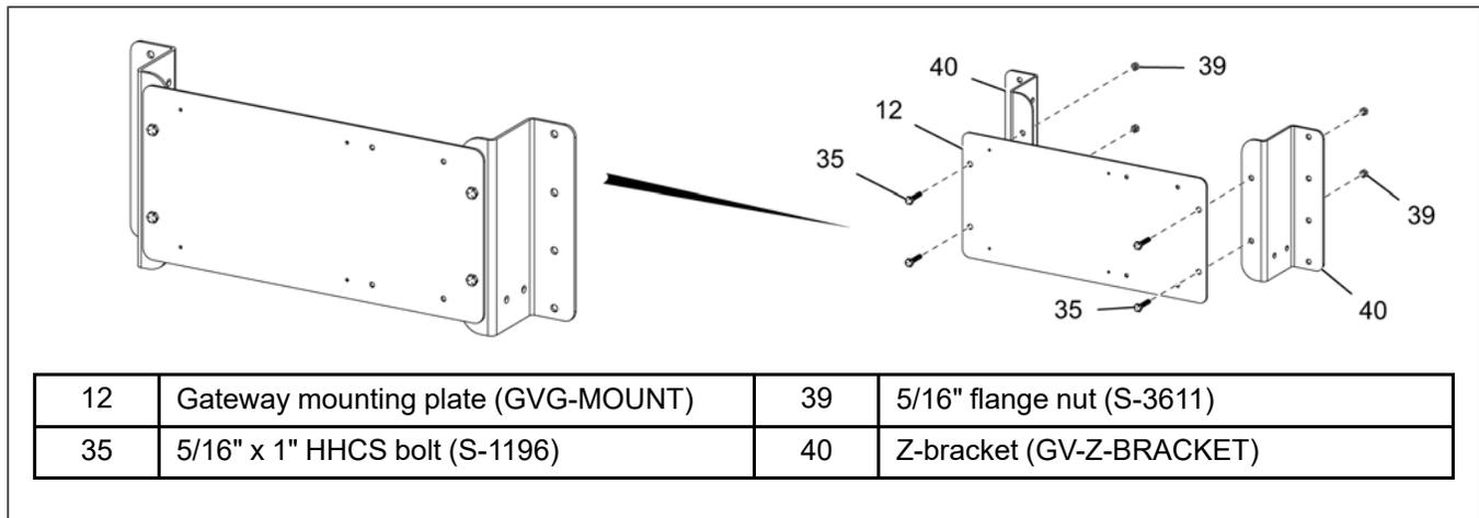
2. Once the appropriate location has been chosen on the bin, level the bracket assembly and line up the holes in the Z-brackets (40) with the peaks of the corrugation of the sidewall (30) and use the supplied 1/4" x 1" self-drilling screws (3) to fasten the assembly to the sidewall (30).
