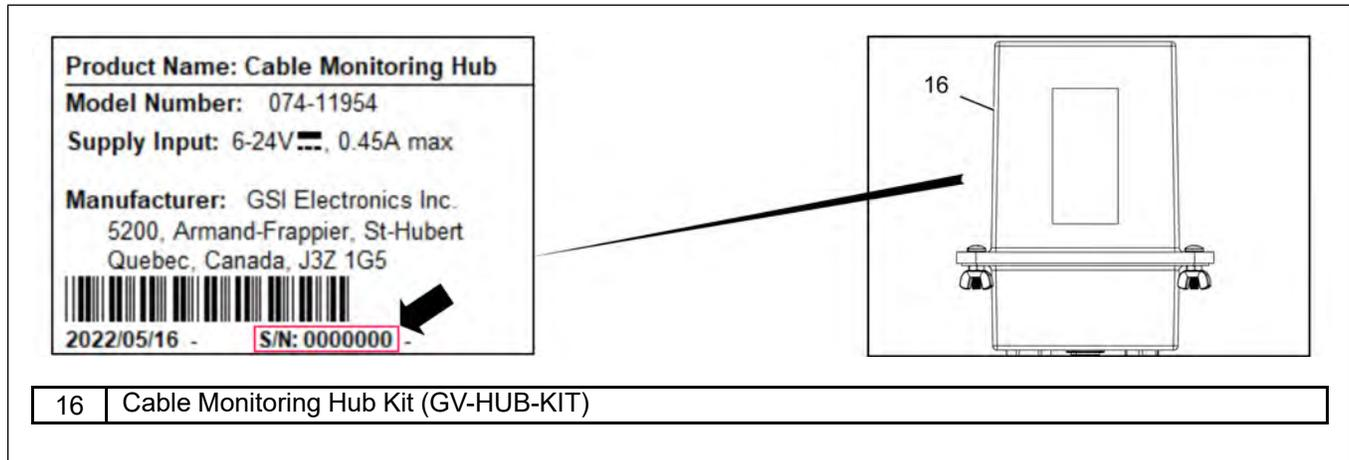
9. The Cable Monitoring Hub(s) (16) will need to be powered after all Lead Wire connections and Fan Control Module cable connections are complete. Refer to [Chapter 7, Activating the Cable Monitoring Hub, page 83](#) for the step-by-step instructions on this procedure.
