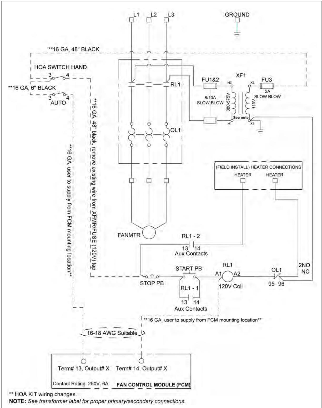
Figure 8-6 480 Volt 3 Phase - 480V control circuit
