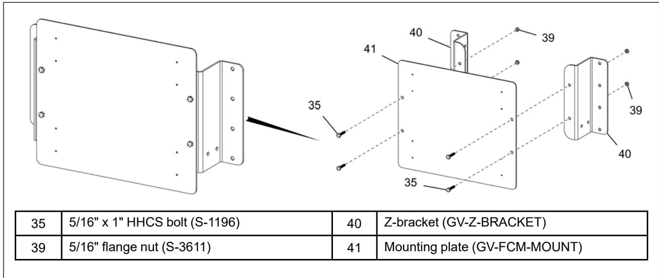
2. At the desired location and at eye level for easy installation, level the bracket assembly and line up the holes in the Z-brackets (40) with the peaks of the corrugation of the sidewall (30) and use the supplied 1/4" x 1" self-drilling screws (3) to fasten the assembly to the sidewall.
