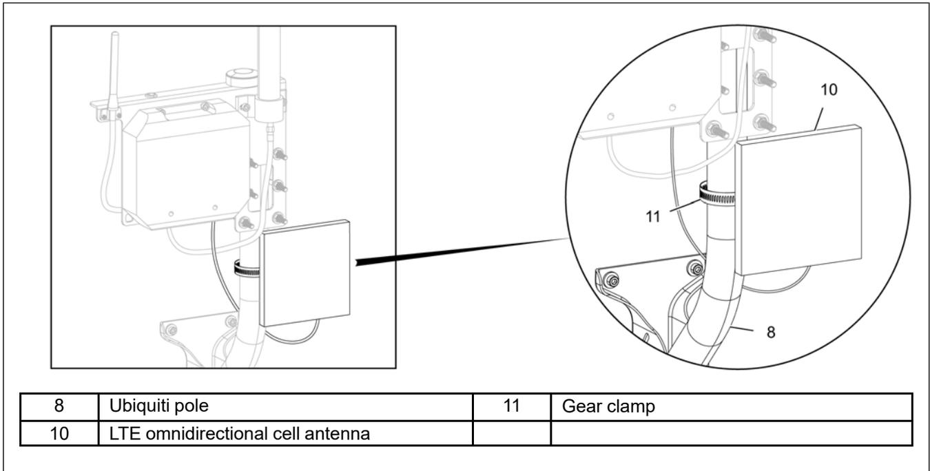
4. Remove the bottom access door of the gateway and connect all installed antennas according to the key below.
