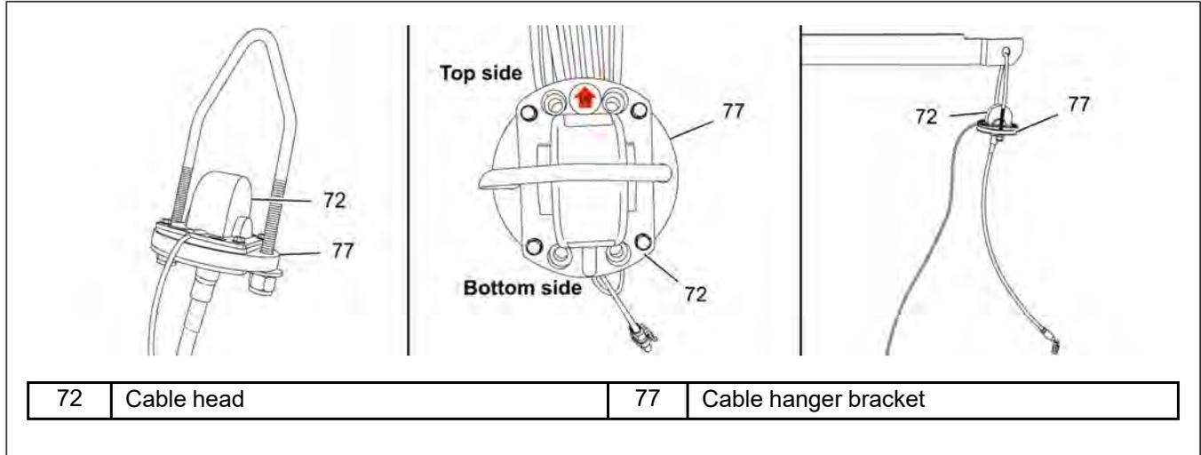
**NOTE:** If installation is being done on an existing bin and access under the roof cannot be achieved, you may install the cable through the bin's heavy peak plate (if applicable) from the outside of the bin as shown in [Figure 4-6, page 36](#). Reach out to a GSI representative if you have questions.
