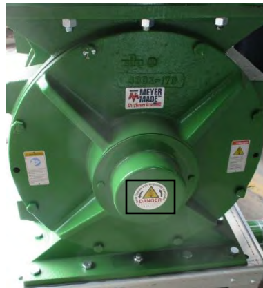
Image 12 – Airlock rotation tag location
