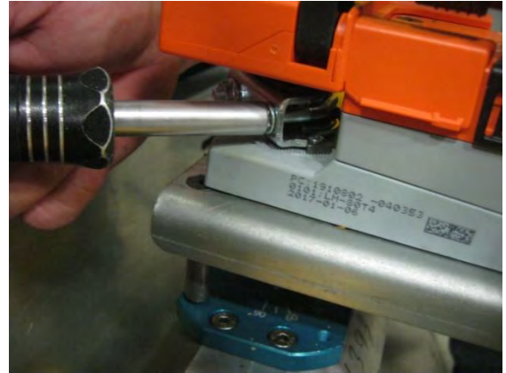
Image 6– Loosening butterfly valve collar
