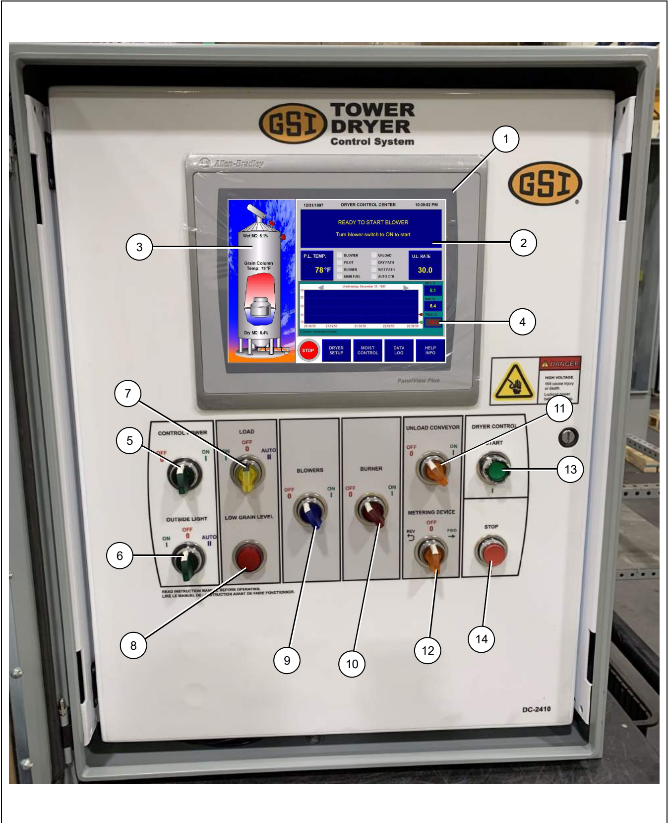
Figure 3B The grain dryer control panel with full color touch screen control.
