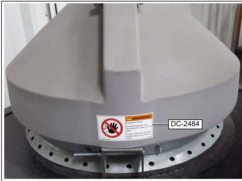
Figure 10E Installing the Decal (DC-2484) to the BFT Lid
