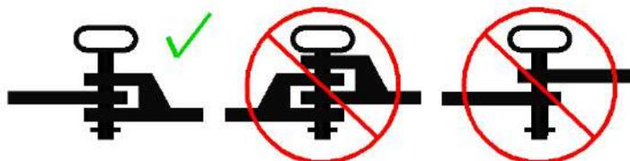
FIG. 2-1. Hitch Connection
