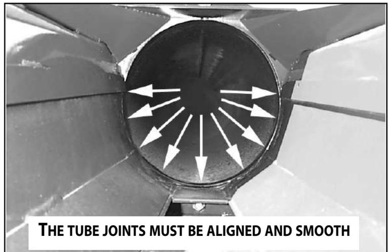
**FIG. 3-5. Tube Joint Alignment**
