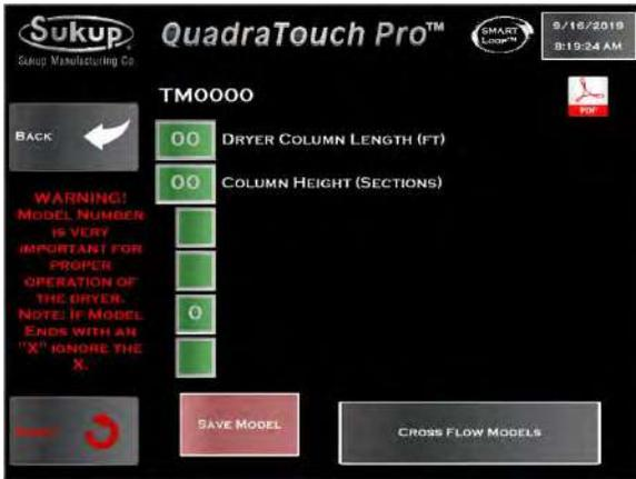
Image at left shows screen for entering dryer length and column height (tiers) for mixed-flow dryers.
