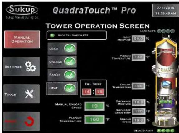
As soon as the unload table has started, any applicable countdown timers will be displayed. Notice the Fill Timer displayed in the bottom center of the screen.
