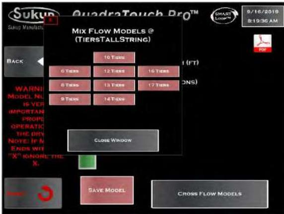
Image at left shows pop-up window for entering number of (tiers) for mixed-flow dryer.
