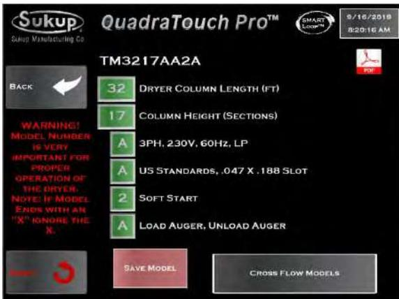
Image at left shows dryer identification screen after entry of all parameters. Press "Save Model" after confirming selections.
