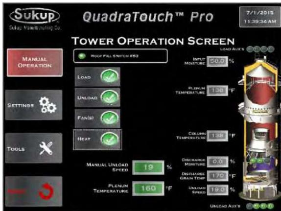
Turning the load, unload, fan(s), and heat on, you can see the devices turning on in order. The fans will start up in sequence along with the load and unload systems. An animated blue flame will show up when the burner control unit senses flame.
