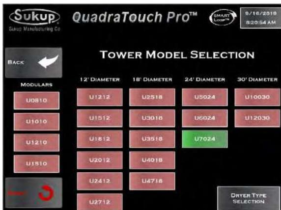
Image at left shows model selection page for tower dryer. Press "Back" after making selection.
