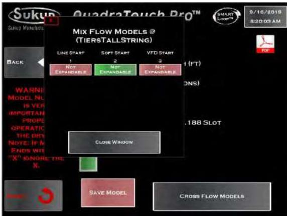
Image at left shows pop-up window for entering start type (Soft start, line start, VFD start) and expandability of dryer.
