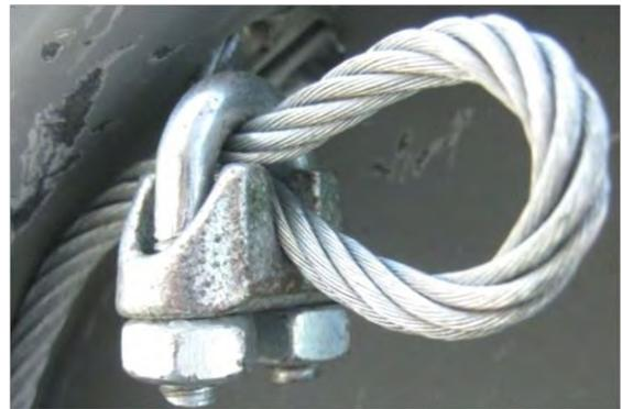
**Image 9 – Folding and clamping cable**
