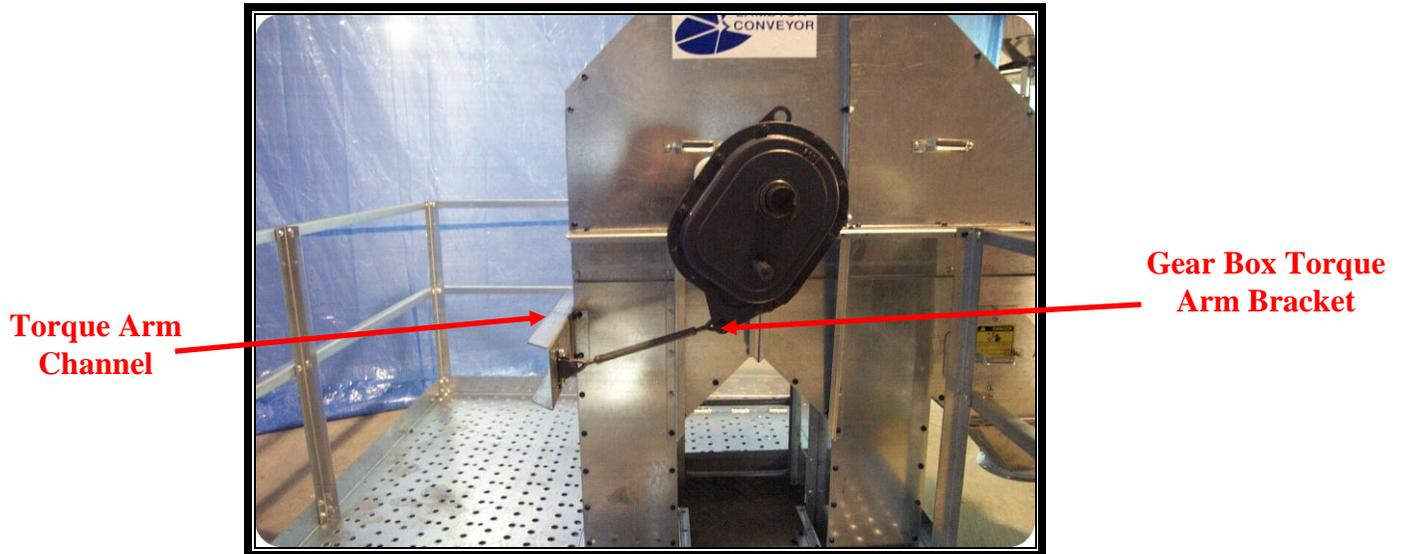
Install the motor(s), sheaves and belts. The smaller sheaves go on the motor(s). Anti-seize compound may be used between the sheave bushing and the shaft it is on, but do not use it between the sheave and sheave bushing as it can cause the sheave to crack. With the motor(s), sheaves, belts, and gearbox installed align the gearbox and (or) sheaves so the belts are running true. Now tighten all components. The threaded torque arm may also now be turned outward to tension the belts.
