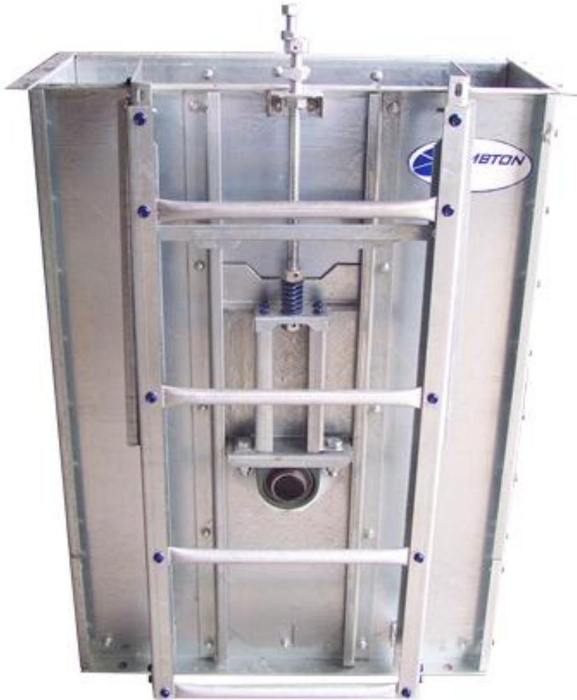
**Note:** to lift the ladder the two top bolts on the ladder main channels are to be removed, then lift the ladder and latch it on a ladder rung further up. For your own safety when the ladder is in the down position be sure to replace the bolts on the ladder main channels, and when not in use place ladder in the upright position. It is the owner's responsibility to ensure unauthorized personnel are unable to access these assemblies.
