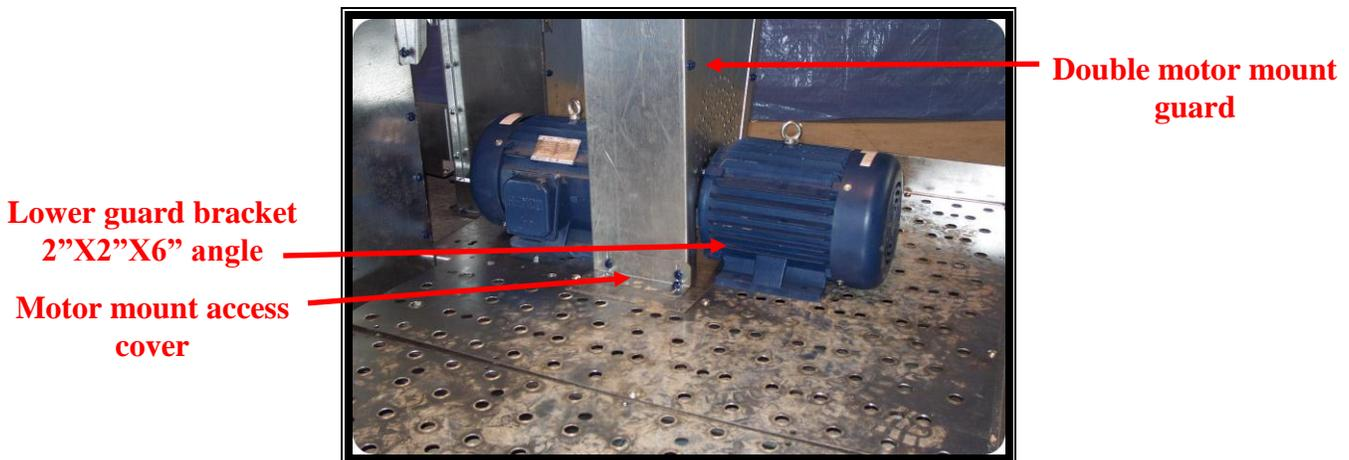
Now bolt the top guard bracket to the guard then to the main bearing channels near the front of the head using  $\frac{5}{16}$ " X  $\frac{3}{4}$ " flange head bolts.
