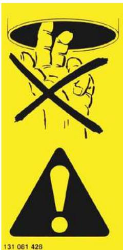
Never put the hand in the outlet of the trough auger, while the cleaner is in operation.
