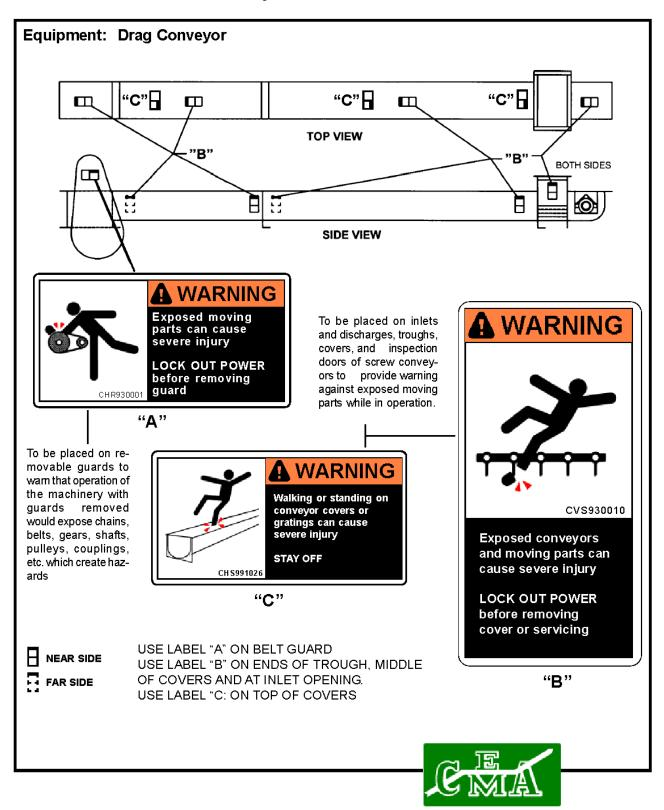
Note: Labels alone do not substitute for a thorough in-plant safety training program centered on the hazards associated with operating your installed equipment. Contact CEMA (www.cemanet.org) or Honeyville Metal, Inc. for replacement labels.
