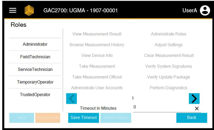
The GAC™ 2700-UGMA moisture tester can create preset lists of permissions which are called 'Roles'. These sets of permissions will allow the admin to define whether a specific operator is able to only conduct a moisture measurement, adjust settings, download new software, all of these, none of these, or conduct other interactions with the GAC™ 2700-UGMA moisture tester.
