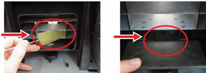
8. Close the trap door and clean hinge under trap door with brush.
