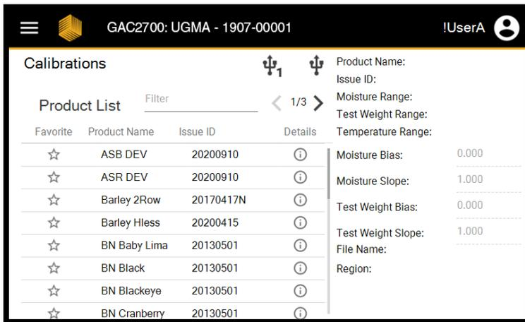
The GAC™ 2700-UGMA moisture tester is shipped with product calibrations that are tied to specific regions of the world. By selecting your region in the Settings, the GAC™ 2700-UGMA unit automatically displays the relevant group of calibrations tied to that region. In many instances, this list includes both Official and Unofficial calibrations:
