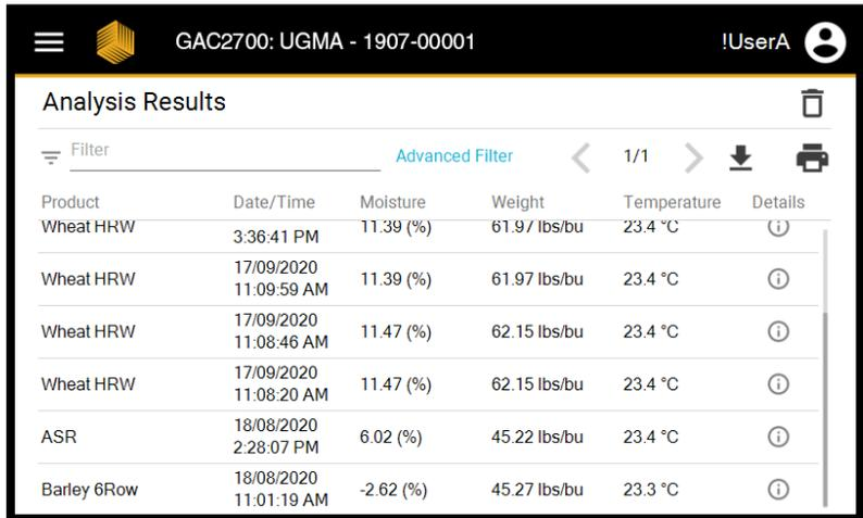
The GAC™ 2700-UGMA moisture tester is equipped with memory to store approximately 3,000 moisture measurement results consisting of all parameters of the measurement. Items such as the grain name, moisture and test weight results, the temperature of the grain at time of measurement, user ID, sample, ID, etc. are all available on this screen.
