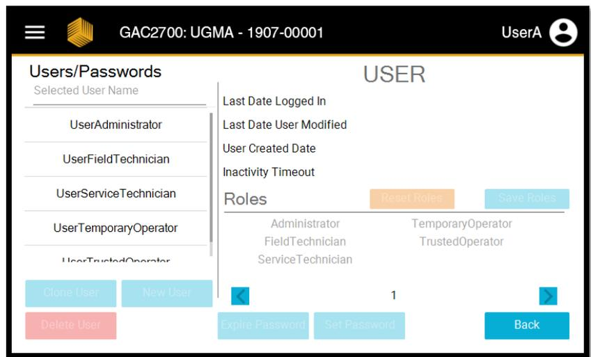
The GAC™ 2700-UGMA moisture tester can be configured for multiple levels of user interaction with the settings that would affect metrology of the instrument. This menu provides the Admin with the ability to configure what pre-defined set of permissions a user would have in the form of roles.
