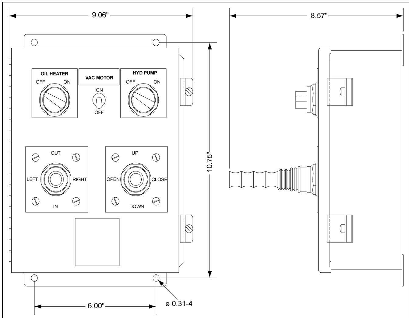
**Figure 6A** Standard NEMA 12 Operators Control Panel Detail
