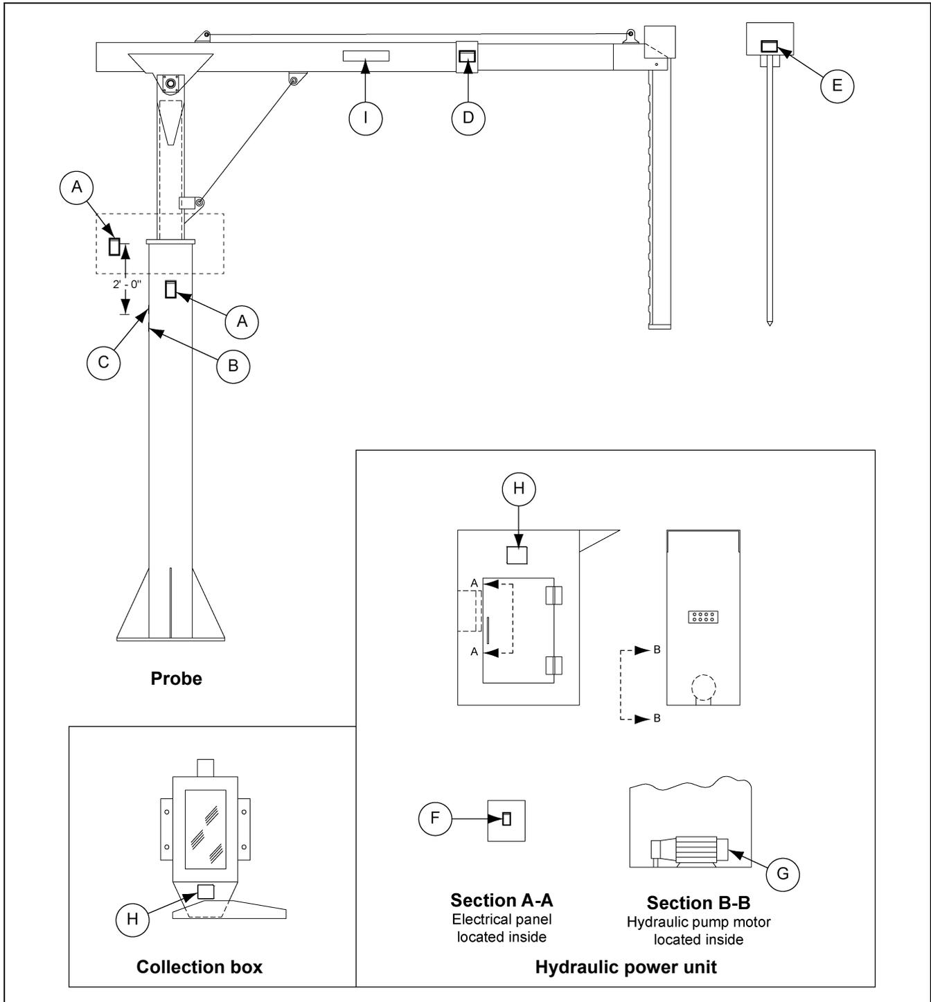
Figure 3A MTP Truck Probe Safety Decals Locations
