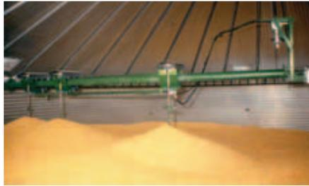
**The Sukup Sweepway™ Power Sweep Bin Unloading System** unloads your grain quickly and is safer, since all controls are located outside the bin, so there's no reason to enter the bin.
